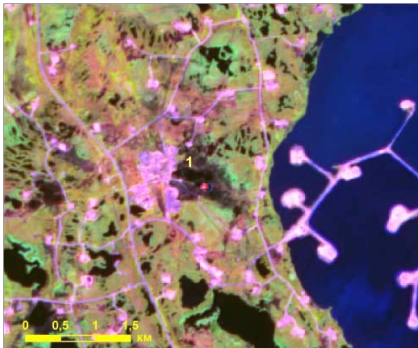
Fig. 5-A. The Samotlor field. Terra/Aster image. Spatial resolution: 15 meters. Date of imagery: July 2, 2002. Scale: 1:50,000. The area contaminated with oil products. Number 1 shows contamination masked by secondary vegetation.
